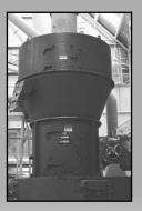
Heavier components; dust-tight gear housings; uniquely sealed, self-contained journal assemblies; cut steel bevel gear drives. Raymond Roller Mills are built to work long and hard under the toughest conditions. That's why many competitive mills that looked tough on paper go to pieces down on the plant floor, while Raymond Roller Mills stay on the job, producing quality product and higher profits for 40...50...60 years and more.
