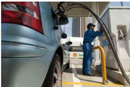
A fuel cell powered car being filled with hydrogen at a station in Tokyo. Courtesy Shell
