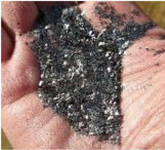
Spherical graphite is manufactured from flake graphite concentrates produced by graphite mines and is the battery anode material (“BAM”) used in lithium ion batteries (“LiBs”). The first part of the process consists of micronizing, rounding and purifying flake graphite to produce uncoated (“uSPG”).
