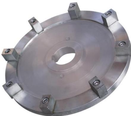
**ACM grinding plate, sharp edge beaters are used for size reduction, round edges for spheronizing**
